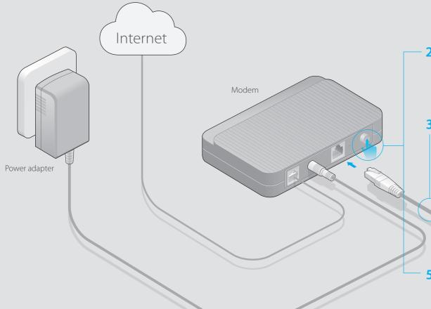
2 Turn off the modem, and remove the backup battery if it has one.
